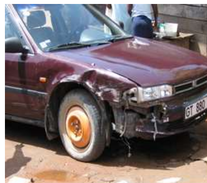
(a) Offside Front Fender Buckled
