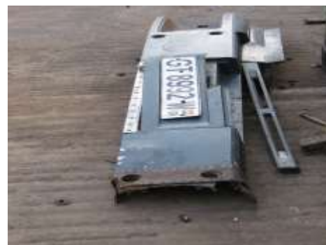
(e) Damaged Front Bumper
