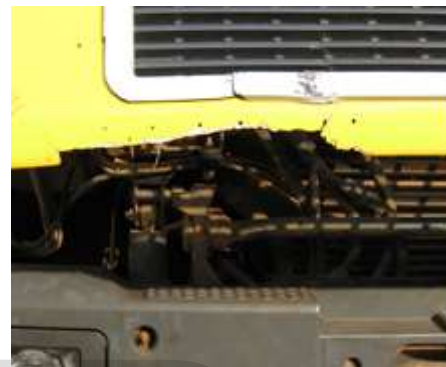
(c) Damaged Bonnet Right Side
