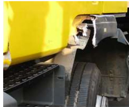
(b) Damaged Stepwell Left
